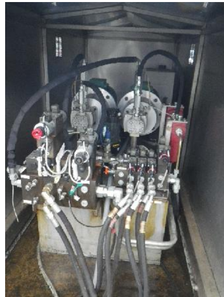
Figure 2-14 : centrale hydraulique
